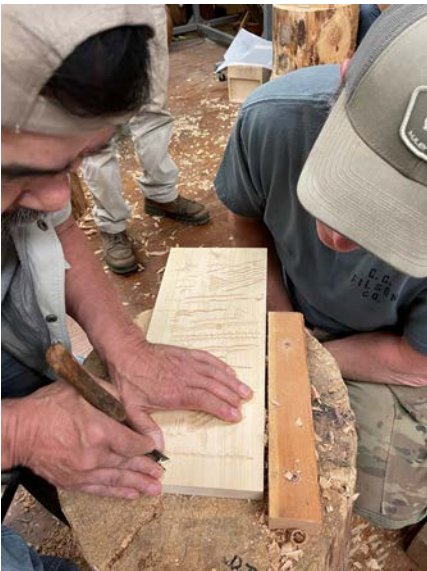
Masa demonstrating his gouges with carved hand-fitting handles for texturing to Adam.
