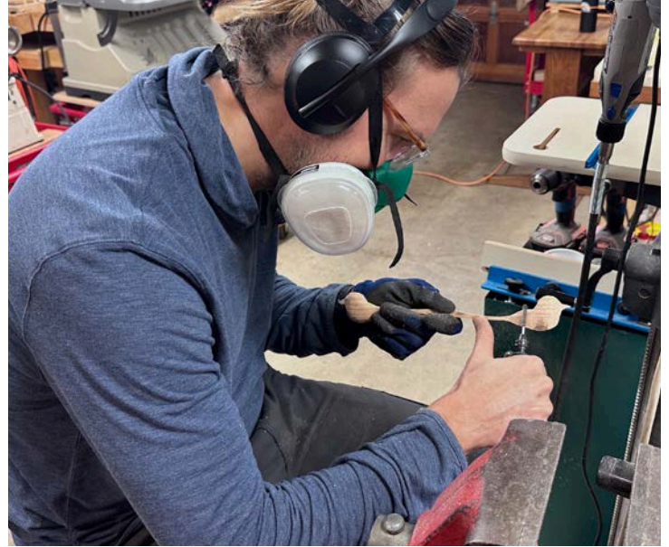
Jeremy Bailey using a Dremel to rough grind a pair of Comfort Birds
