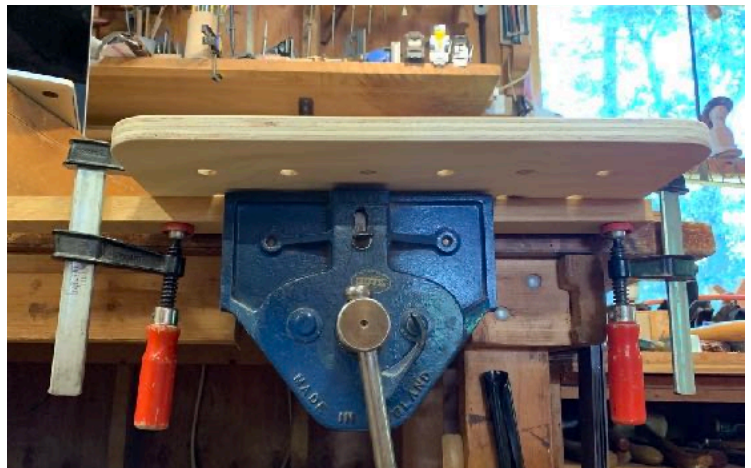
Fig 2 - This view shows the plate clamped to the batten which is held in the front-vise
